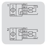
This capacitive level sensor is pre-adjusted for the detection of bulk materials or liquids with a dielectric constant  $\varepsilon_r$  of 2 to 80.
